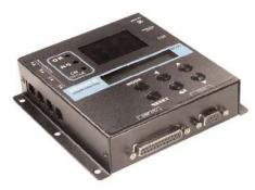
Scout screw counter helps manufacturers detect and eliminate costly screw-fastening errors during the assembly process. Using a screw counter is like putting the eyes and ears of a quality control manager where they are needed most - right on the assembly area. The scout is designed to detect cross threading, omissions, unfinished rundowns and cycle complete. The screw counter takes the control of the assembly process out of the operator's hands.
