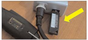
To adjust the settings the Program Lock Key must be is plugged into the STC40 Transformer.
