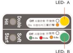
The clutch of the electric driver works twice at the set torque under the "Double Hit" mode. The Double Hit will increase the repeatability accuracy at the target torque by double checking.
